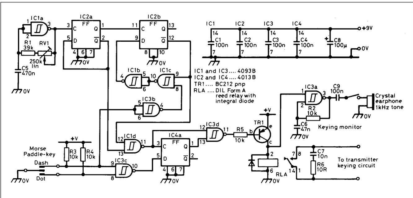
Fig 18.5: The G3BIK simple keyer uses four ICs for precision Morse
