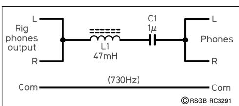
Fig 18.7: Circuit of the two-component CW filter
