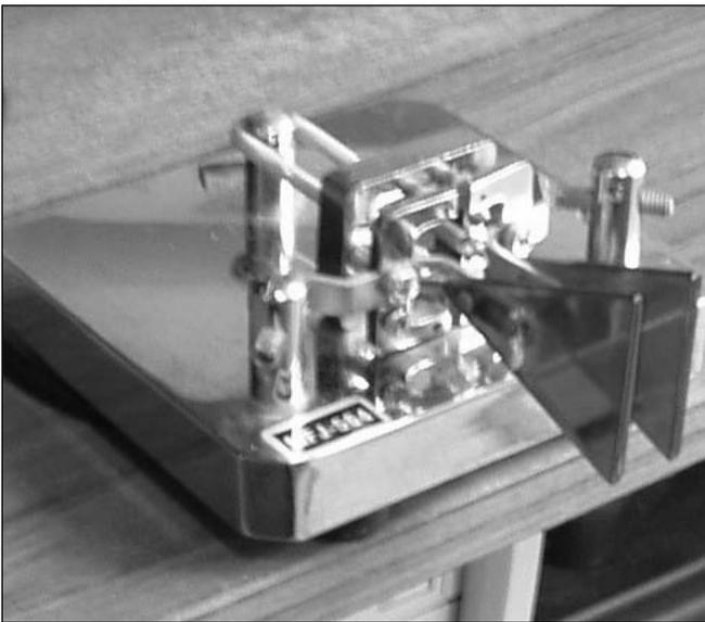
Fig 18.4: A paddle for use with an electronic keyer
