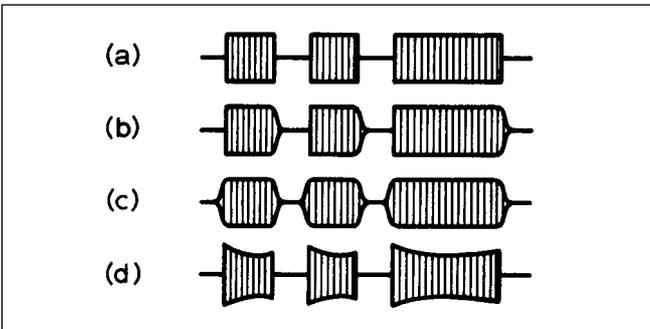
**Fig 18.9: Keying envelope characteristics. (a) Click at make and break; (b) click at make with click at break suppressed; (c) ideal envelope with no key clicks; (d) affect on keying envelope of poor power supply regulation**
